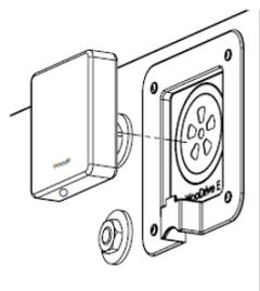
Figure 6: Inserting a portable battery.
